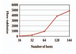
Fig. 1: ECMP flow table size according to different number of hosts.
