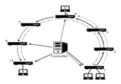
Fig. 3: Host B communicates with Host A, in 4 hops linear topology, and Host C communicates with Host D in 12 hops linear topology.
