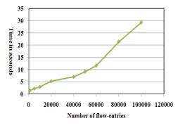
Fig. 2: The response time of flow status requests according to different flow table sizes.
